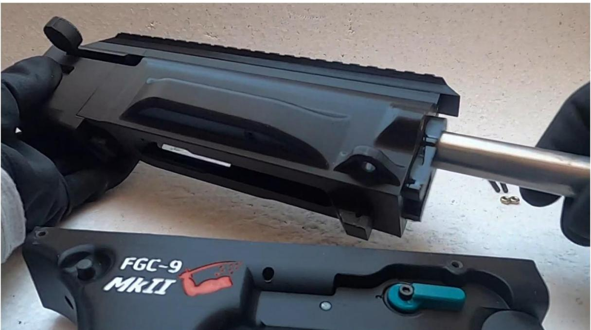
If you have silicone spray on hand, spray it on the side and bottom surface of the bolt assembly.
