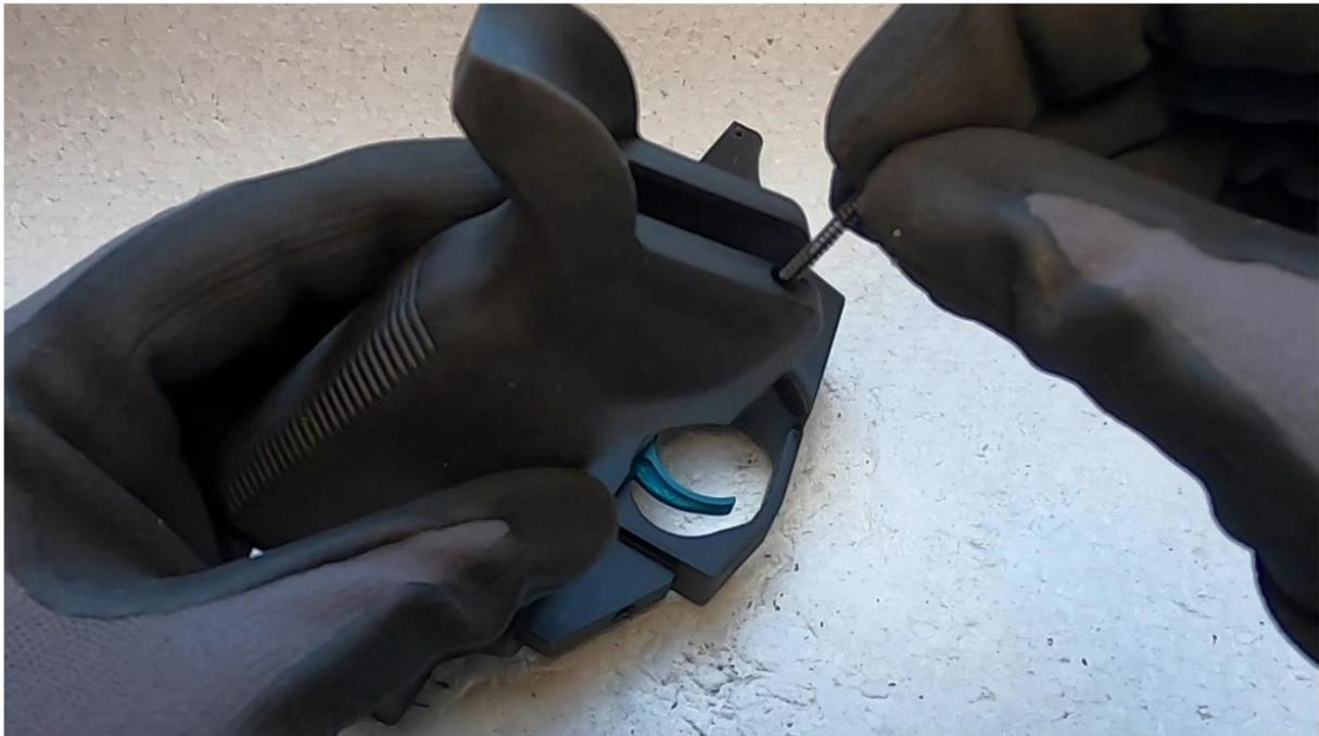
Take the fire selector detent spring and put it into the dedicated hole inside the top of the pistol grip.
