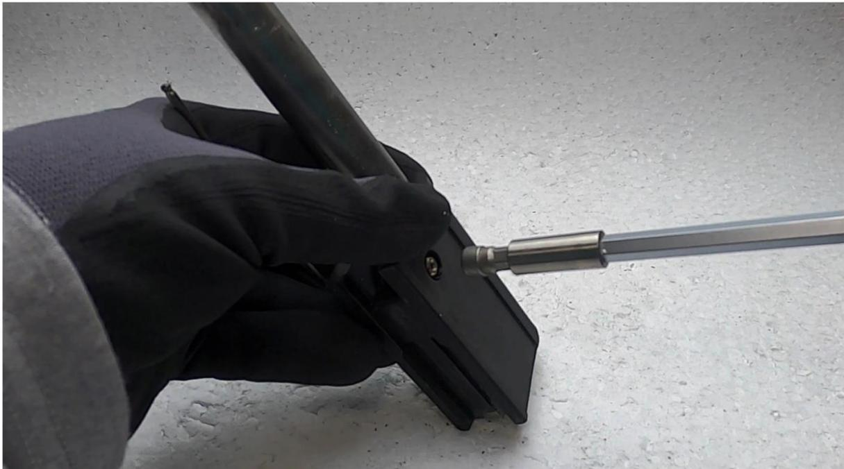
While making sure that the bolt assembly does not fall out, tip the bolt assembly with the bolt face down and push against the back of the firing pin with your finger and insert the 20mm M3 socket head screw into the small hole on the left side of the bolt.
