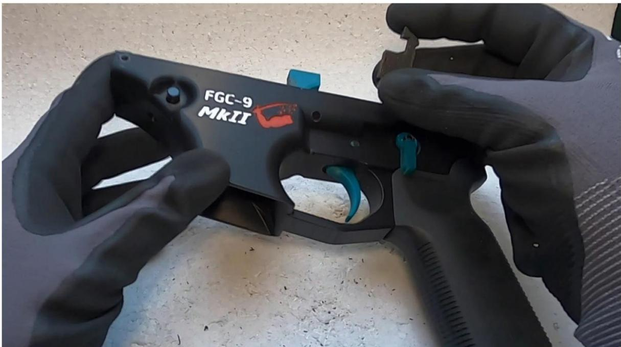
Take the magazine catch bar and push it into its cavity against the spring pressure of the magazine catch spring and try to align the hole on the bar with the hole on the lower receiver.
