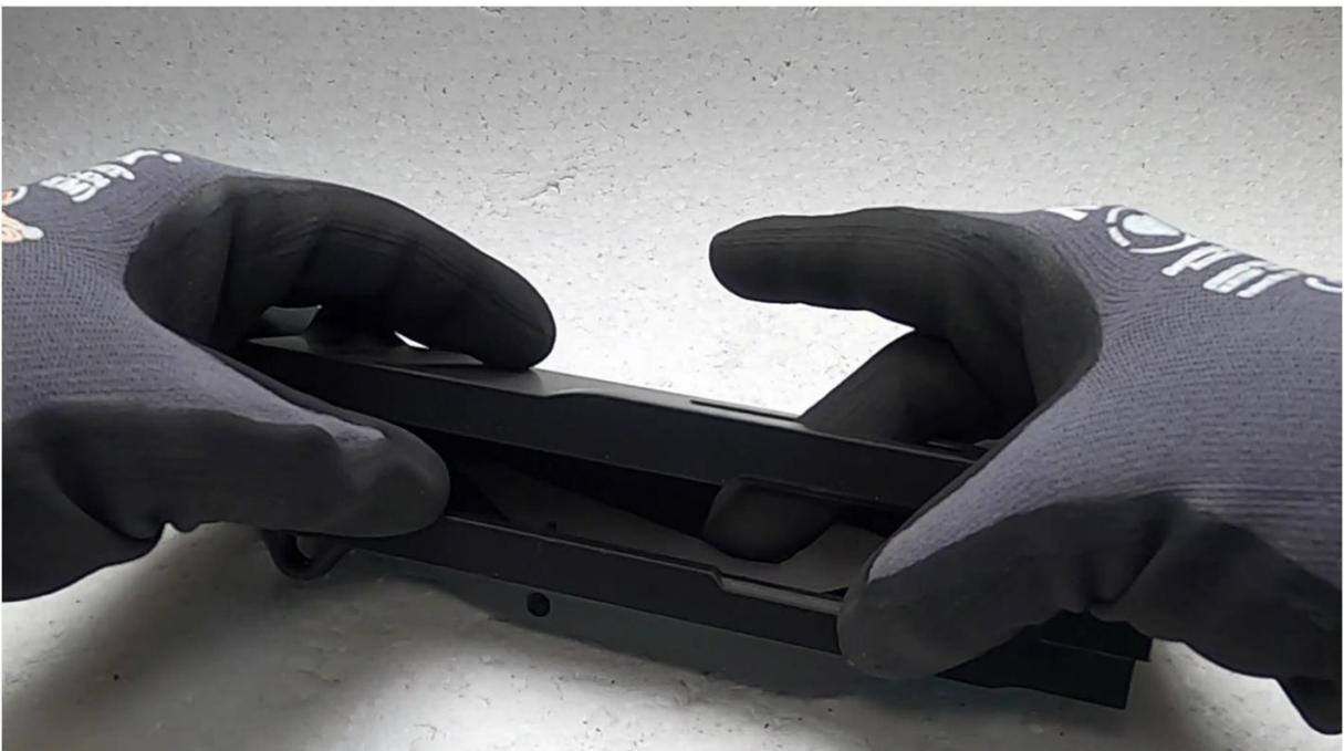
Take the ejector and try to get it into its designated slot on the inside of the upper receiver. Make sure to put it in there in the shown orientation.
