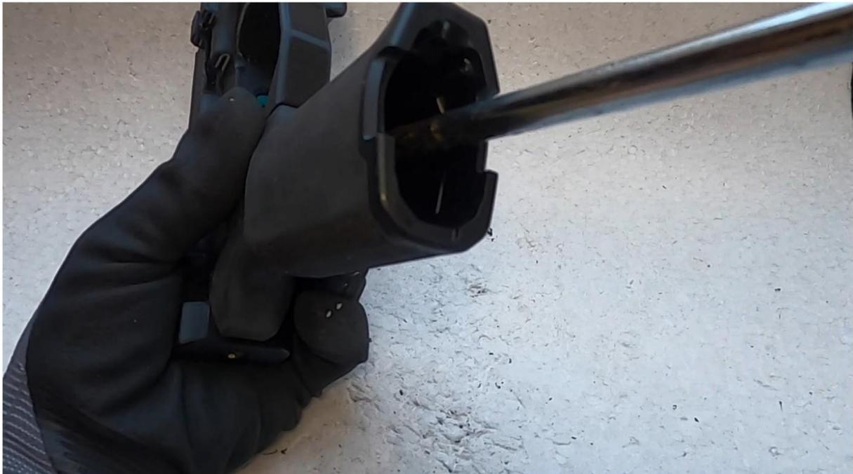
While making sure the fire selector is in the position mentioned previously and the fire selector detent still inside the hole, push the pistol grip onto its mating surface and make sure the fire selector spring goes against the bottom of the fire selector detent.
