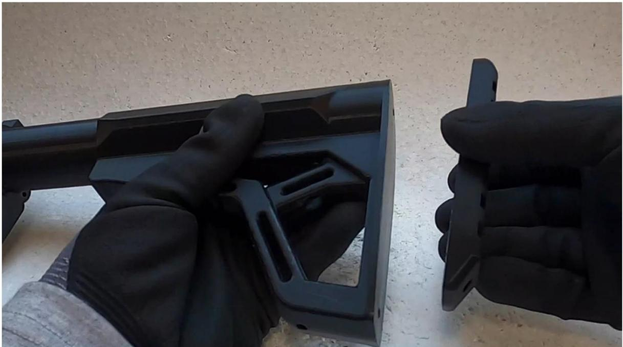
Making sure that the M4 screw is properly in place as you can see from the top picture, take the butt plate and hold it against the end of the stock.
