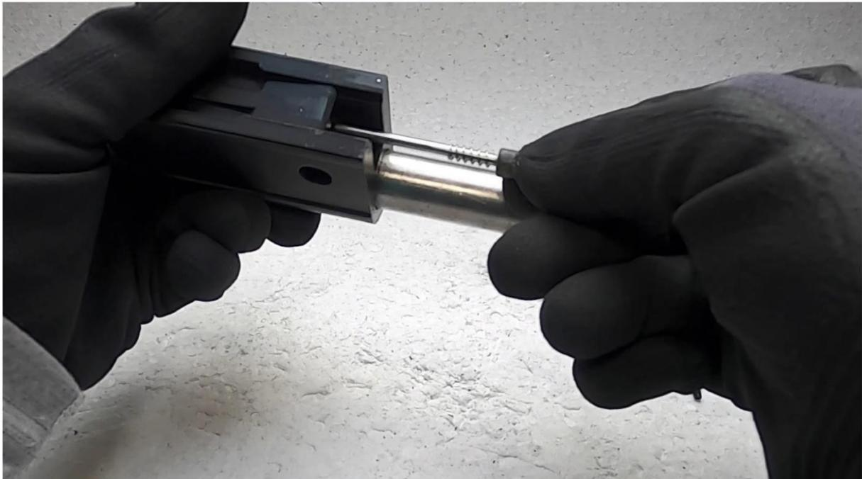
Take your firing pin spring and shove it onto the firing pin.
