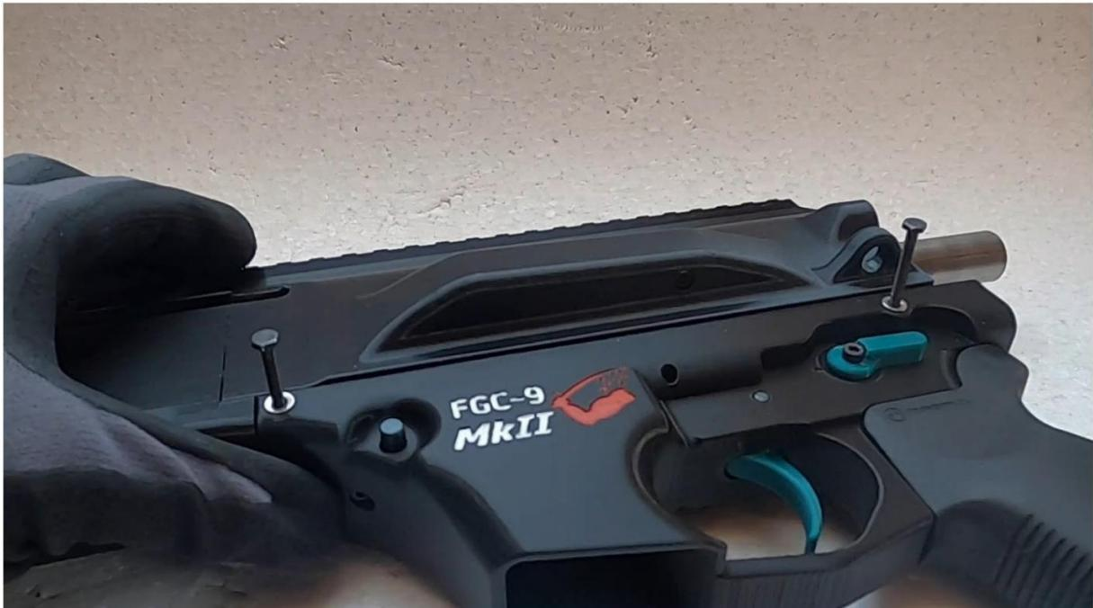
Pull the bolt assembly slightly out of the upper receiver, as to make sure that you have room near the chamber area of the upper receiver. This will make sure you can mate the lower receiver against the upper receiver and prevent the feed ramp from bumping into the bottom of the bolt.
