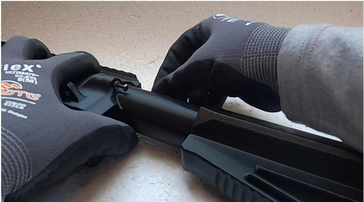
Now push the stock assembly against the back end of the main assembly and secure it with the 4x 20mm M3 hex head screws making sure you include 4x M3 washers.
