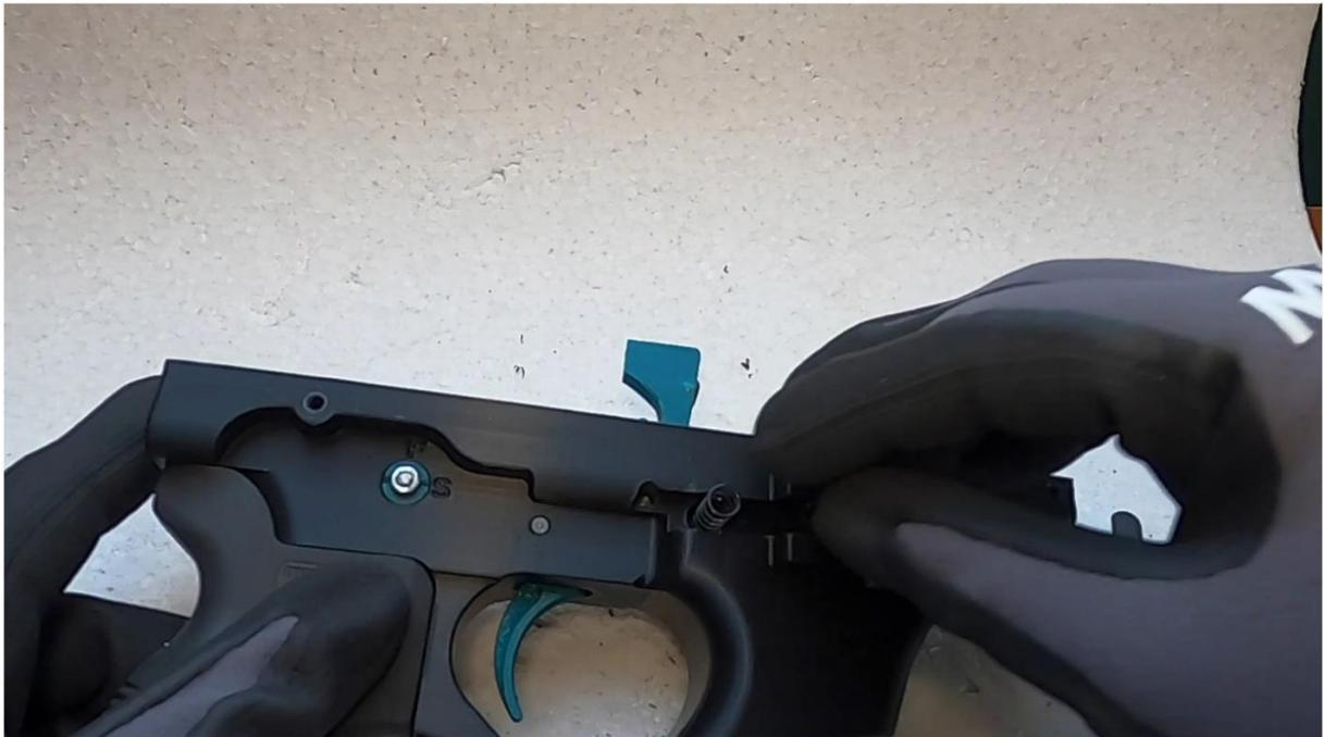
Insert the magazine catch button into the hole you see in upper picture.
