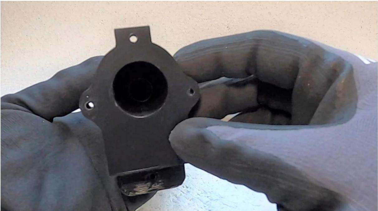
Insert the secondary buffer spring into its dedicated slot at the bottom of the buffer tube. When you printed the buffer tube a piece of support that looks like a rod should have been left. Use that rod piece to push the secondary buffer spring firmly into place at the bottom of the buffer tube. To make sure it is firmly in place, try to shake out the buffer spring.
