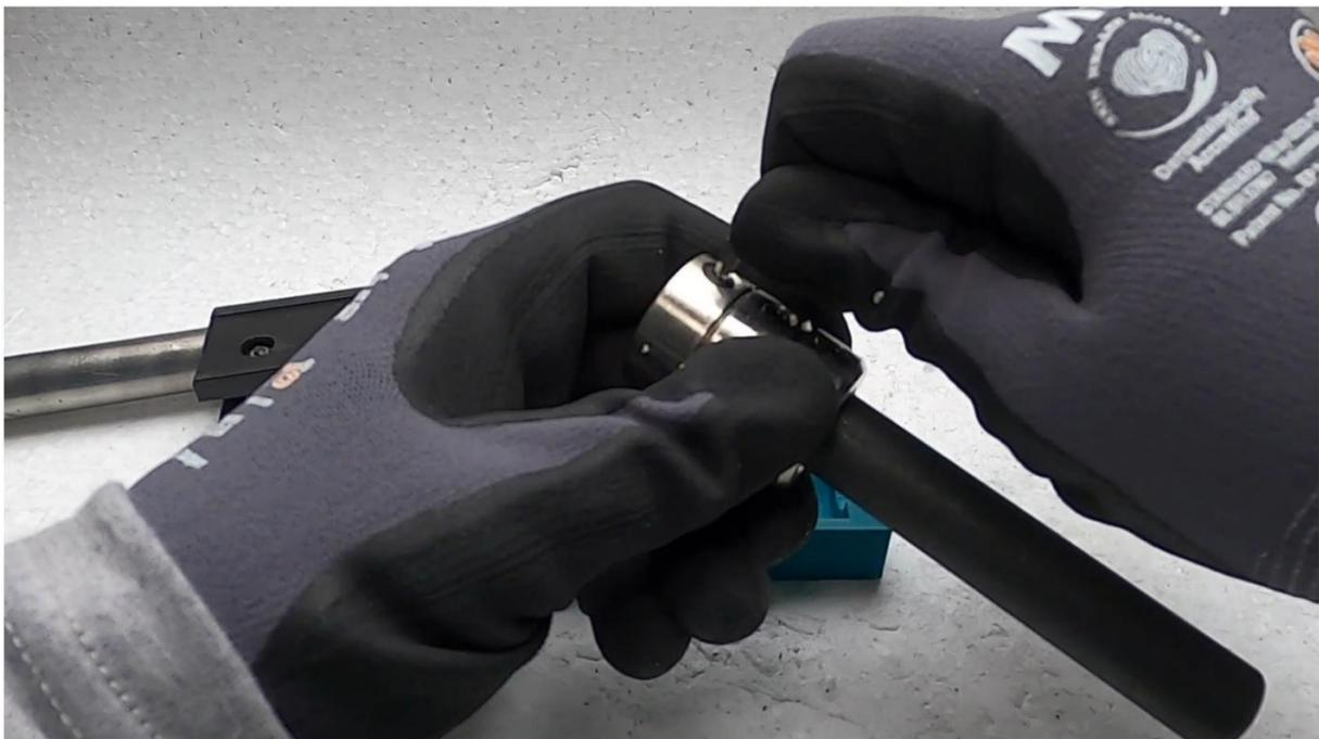
Being extremely careful that you don't move anything apart from the bolt assembly, slide the bolt assembly out of the setup and immediately tighten the grub screw of the center shaft collar.
