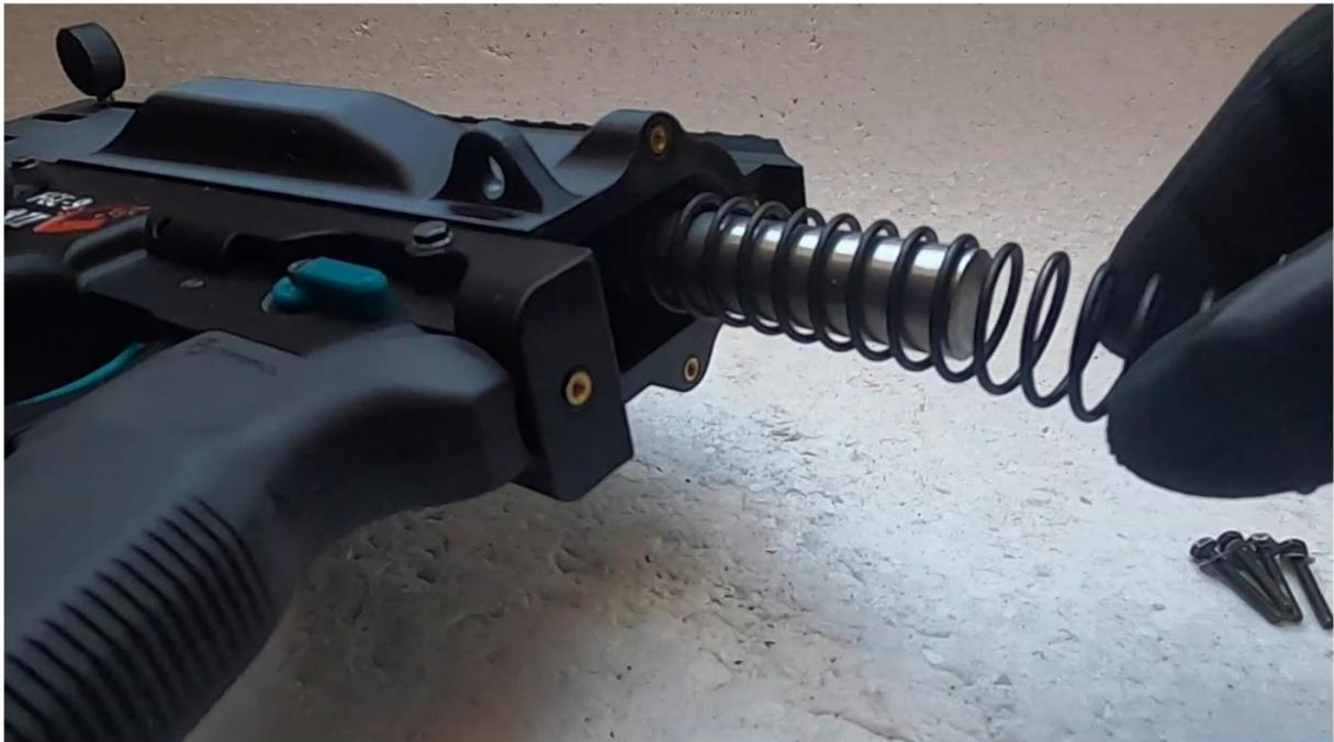
Once you were able to align the holes, you can insert your last two 40mm M3 screws, along with M3 washers from one side of the lower receiver and then secure them on the other side with M3 nuts.
