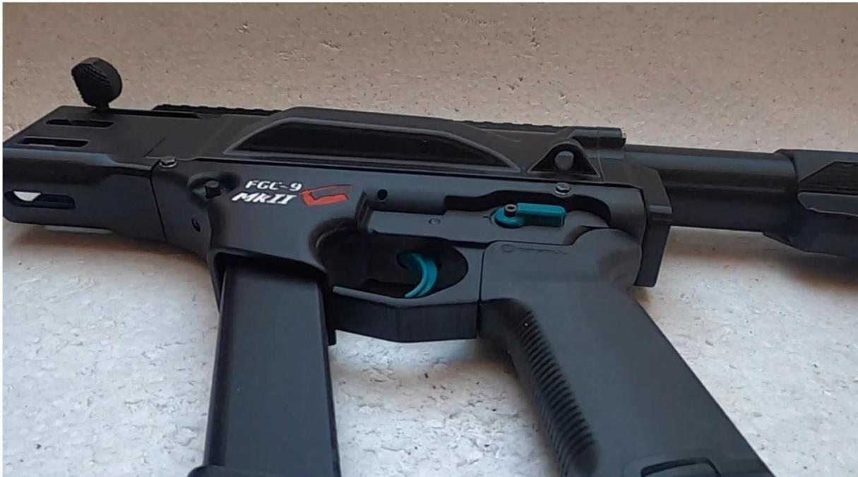
Make sure you push the stock assembly firmly against the backside of the main assembly while securing each screw. Not doing so may cause unnecessary stress to the first two or three screws as are securing the last ones. So make sure after you started screwing in the first screw, to constantly hold the stock assembly against the main assembly while screwing in the rest of the screws.
