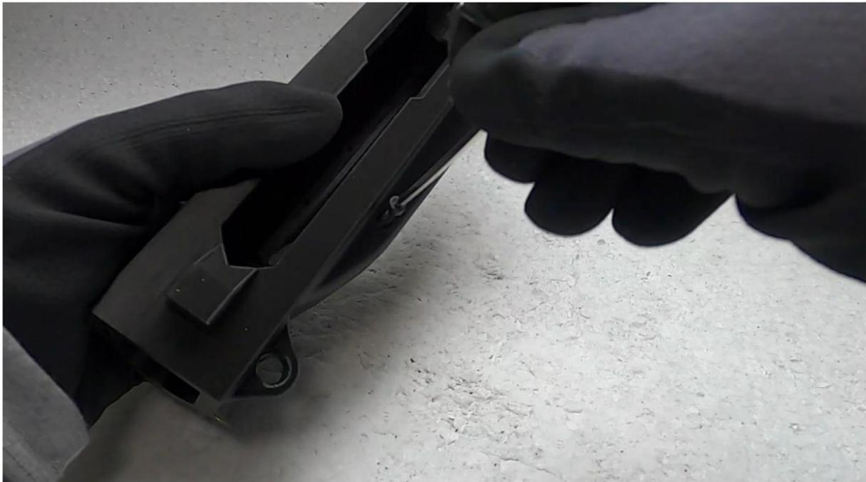
Align the hole on the ejector with the hole on the underside of the ejector cavity and screw the Socket Head Screw M3,16mm into place with the appropriate Allen key.
