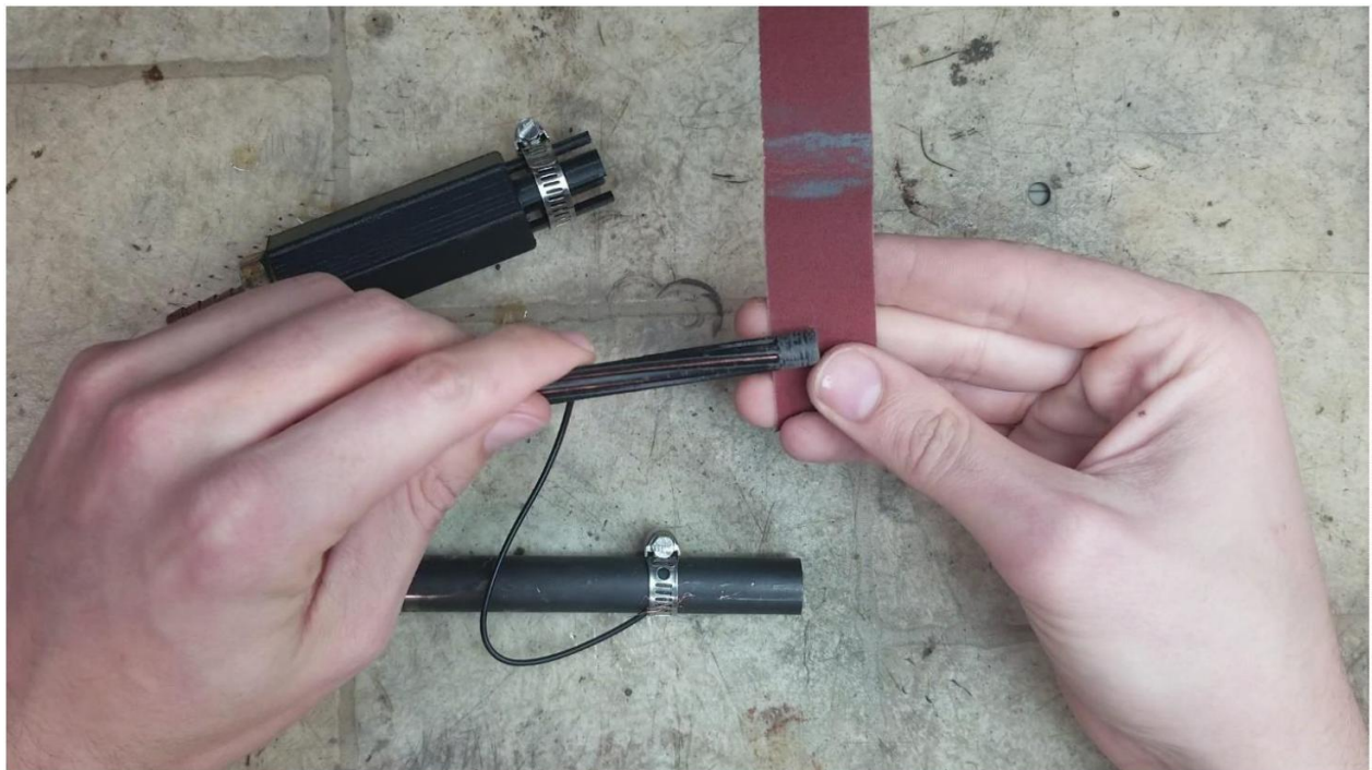
Sanding the end of the mandrel to ensure a smooth fit
