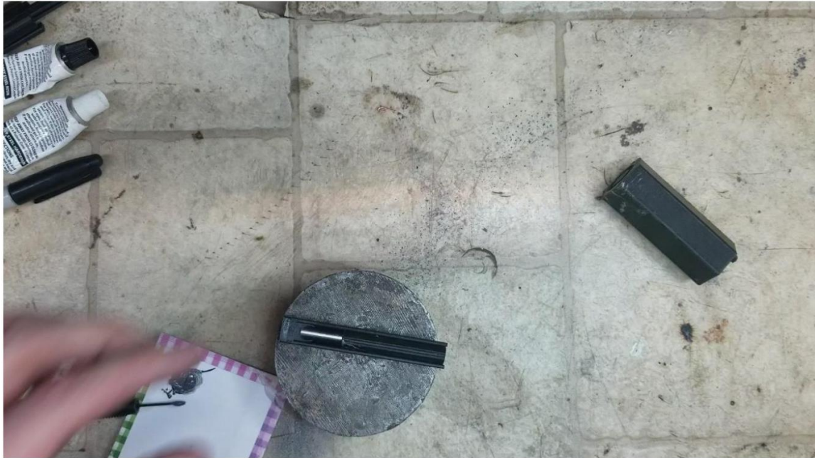
Rod fully pushed inside of jig. Note that this should be done with the jig upright on a flat surface.
