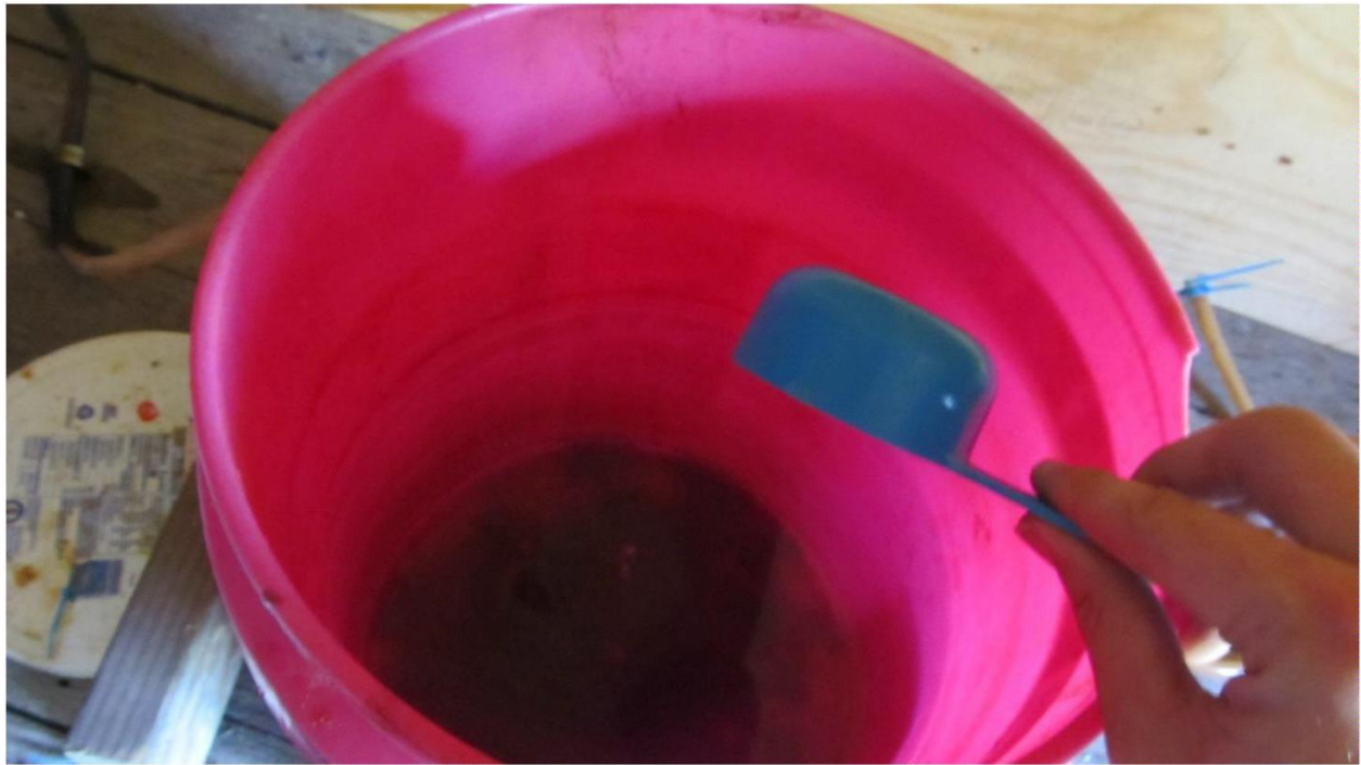
Step 3: PREPARING ELECTROLYTE - Pour your salt into the reservoir. Mix it in.
