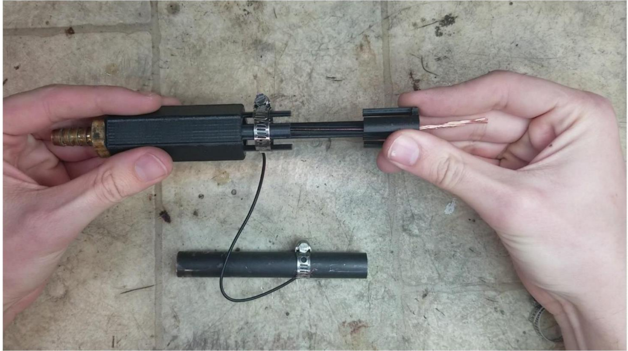
Checking the fit between mandrel and fixture
