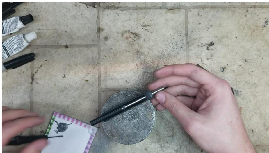
Push the rod down from the top and into the insulator (which is sitting inside the jig)
