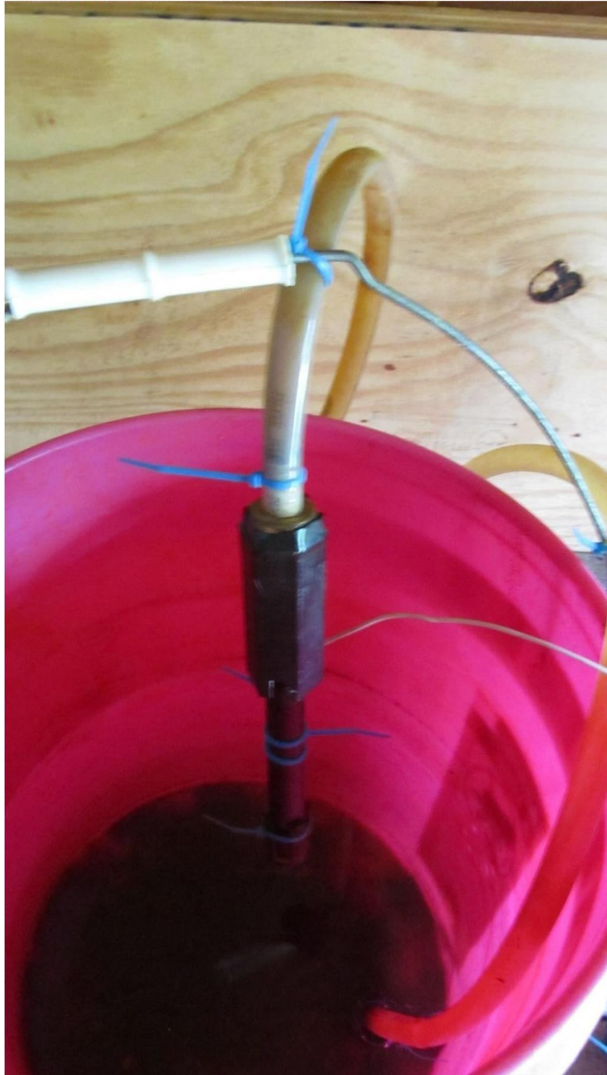
Step 17 continued: MOUNTING THE TOOLHEAD – example picture showing the toolhead hanging above the bucket. Note position of zip ties – these zip ties can all be used interchangeably with hose clamps.
