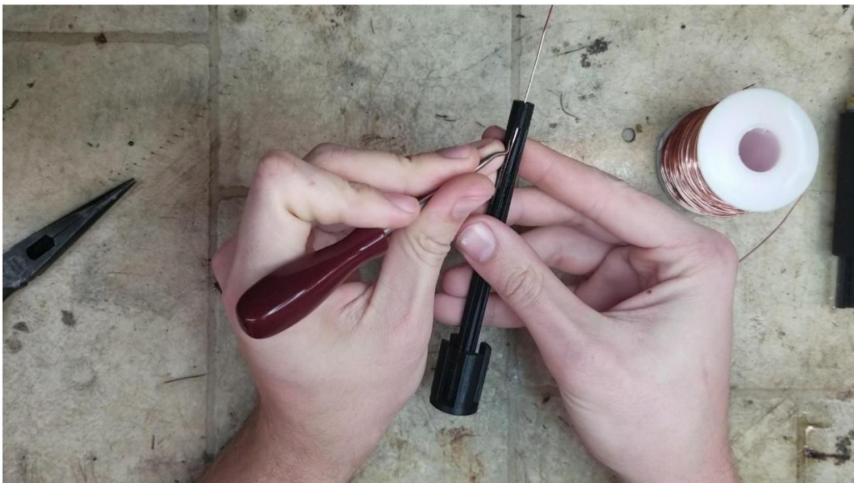
Pushing the wire down into the slot might be required when starting the wire. It should push in easily.
