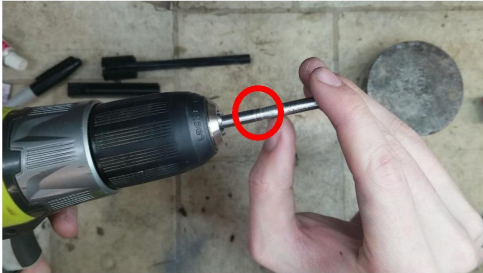
Note the shoulder formed on this rod at the 1.2" mark
