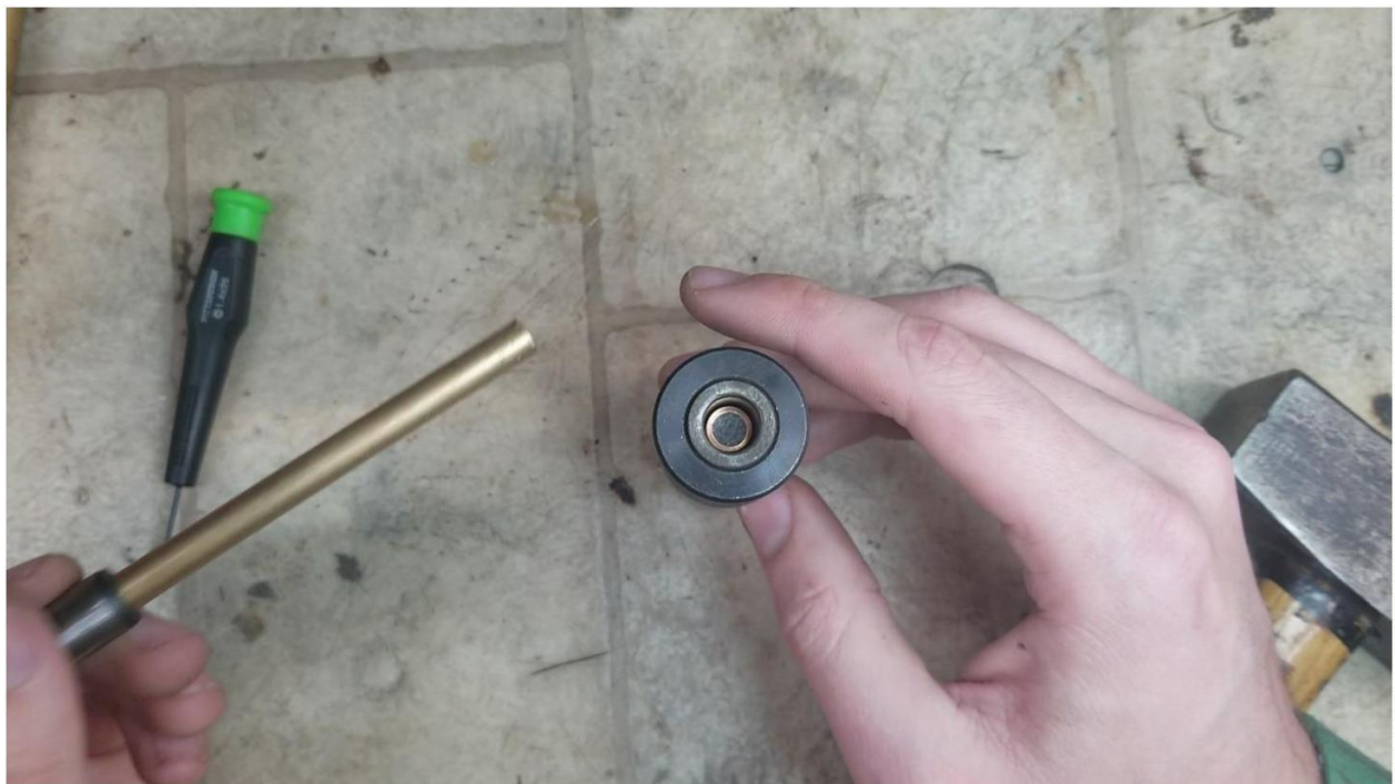
Example punch used to hammer the bullet down the barrel.
