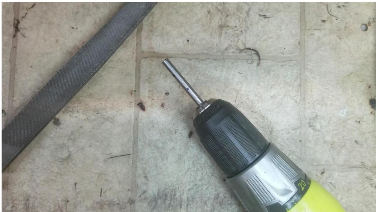
Rod chucked up in a drill. Note the two marks placed on the rod, one at 0.57" from the end, another 1.2" from the end.
