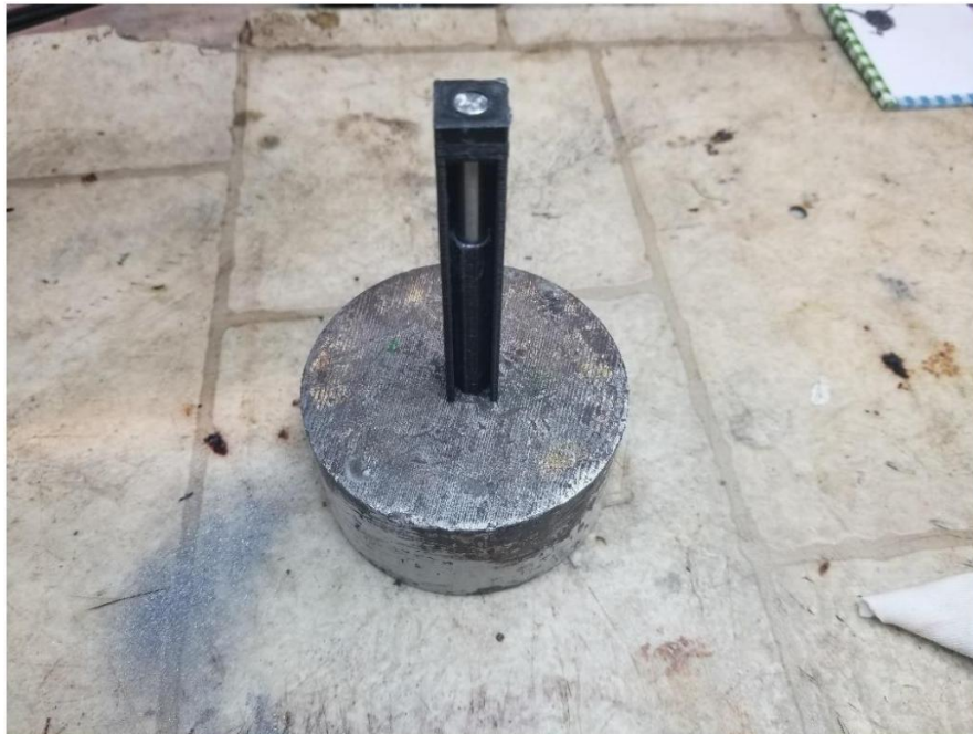
The assembly upright on a flat surface. Note that the rod is pushed flush with the top of the jig, the assembly is on a flat surface.
