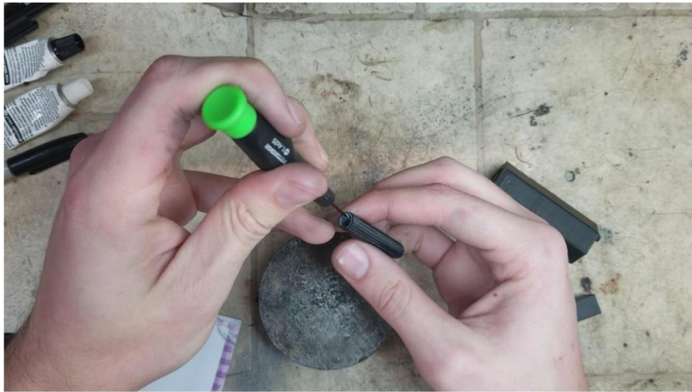
Apply a little JB weld to the inside of the mouth of the chambering tool insulator
