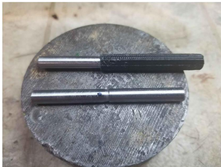
Tapered rod (bottom), tapered rod inside it's insulator (top).
